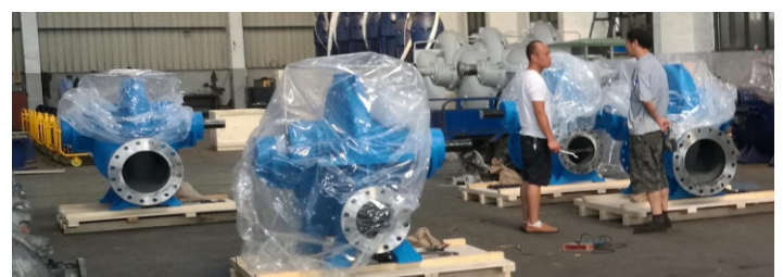
AURUM PUMPEN duplex stainless steel split casing pump ( BHS250-800, BHS300-700 )
